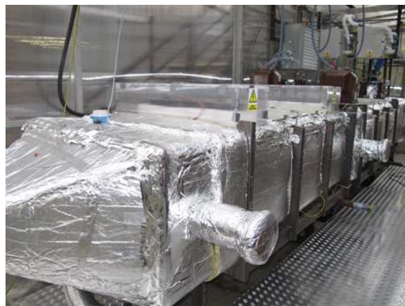
Figure 4. Photograph of experimental channel. In foreground is the one-stage electrostatic precipitator and at the background, the charger/agglomerator
