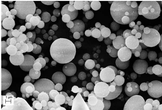
Figure 5. SEM micrograph of fly-ash particles used in the experiments (SEM Zeiss EVO 40)
