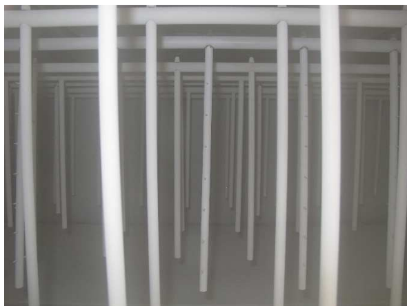
Figure 3. Electrodes of experimental agglomerator (covered by fly-ash)
