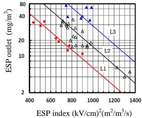
Figure 1. ESP outlets via ESP index
