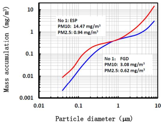
Figure 6. PM<sub>10</sub> emission at ESP and FGD outlets
