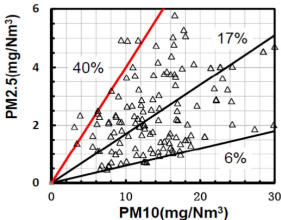
Figure 7. PM<sub>2.5</sub> via PM<sub>10</sub> at ESP outlet
