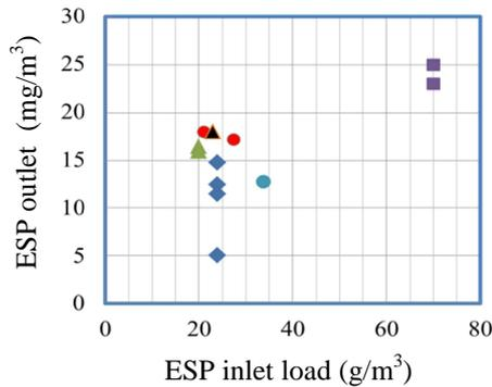
Figure 2. ESP outlets via inlet load
