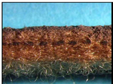
Figure 14. Cross section through exposed needle felt from FF pilot plant in Belgium
