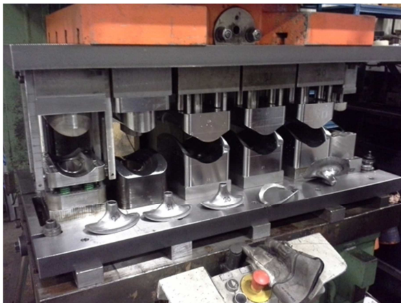
Figure 7. One of the stamping tools for production of radius nozzles
