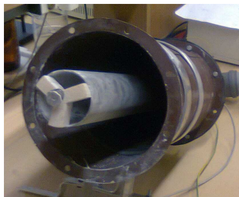
Figure 3. The photograph of one end of the electrostatic precipitation part of the cyclone
